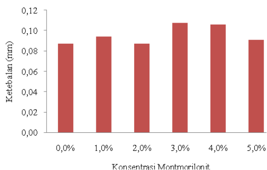
Gambar 3. Ketebalan Edible Film Komposit Karagenan-Montmorilonit
